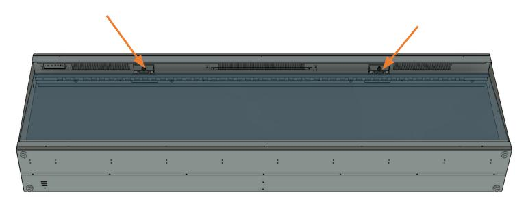
Unscrew the bolt and hinge holding the front glass.
