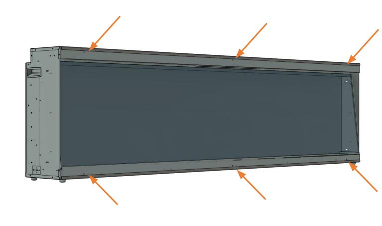
With the front trim removed, ensure the magnets and holders are removed from the top and bottom trim
