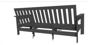
Install "Y" brackets to the outside of seat and back supports. Screw into side and also into back.
