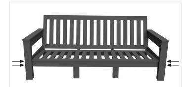
**6** Insert screws on side legs (2 screws per side where the holes are).
