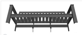
Install rear leg support with 2 screws.
