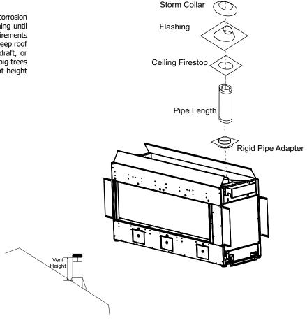
When using Rigid Vent other than Simpson Dura-Vent, 3 screws must be used to secure rigid pipe to adaptor.
