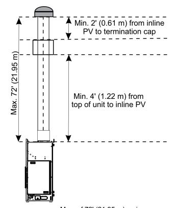
Max. of 72' (21.95 m), using up to six 90° elbows
