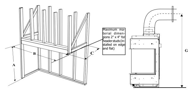
Note: This appliance must be installed on a level and solid surface such as a plywood floor which must be the full width and depth of the appliance.
