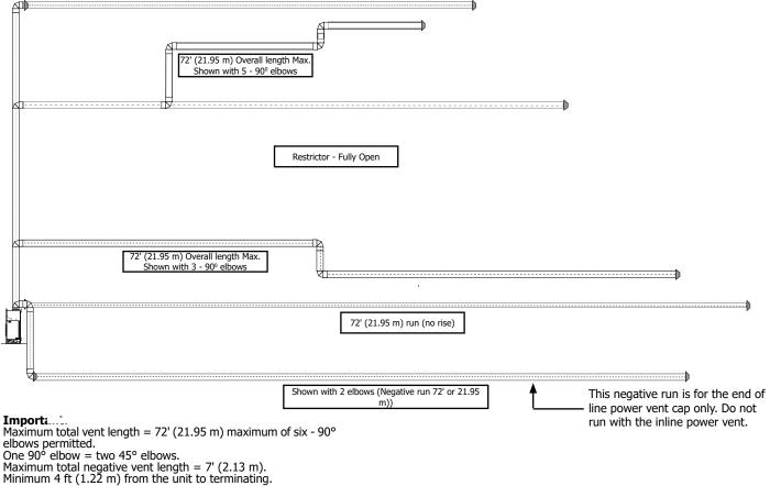
Note: Maximum length of 72 feet (21.95 m) is based on overall length of combined chimney components.
