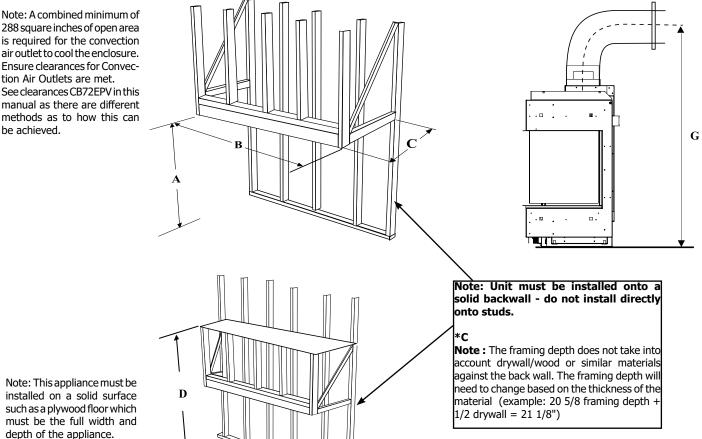
installed on a solid surface such as a plywood floor which must be the full width and depth of the appliance.
