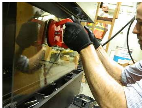
Handle front panel with supplied vacuum clamps
