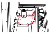
Remove 16 screws securing valve tray
