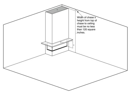
Note: The ventilation opening may only be placed above, on side/front and in front as shown above and on the next page. Ventilation grills can never be placed behind the appliance.
