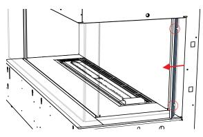
Loosen 2 screws from inside the firebox to remove the side drywall trim pieces
