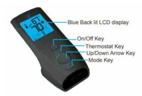
Figure 1: Proflame Transmitter
