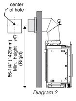
7. Ensure that the pipe clearances to combustible materials are maintained (Diagram 3). Install the termination cap.
