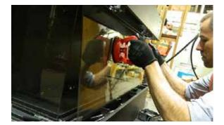
Handle front panel with supplied vacuum clamps
