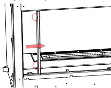
4. Loosen 2 screws from inside the firebox to release the existing side drywall guide, remove guide and recycle.
