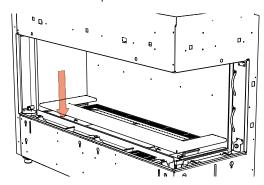
2. Install panel clips into the slots at the top of the back panel as shown.
