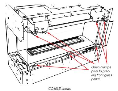
6. Lift up the front panel using the supplied vacuum clamps and position into the lower front channel—ensure the front panel is accurately centered—with the front panel in position—secure in place by closing the 3 lower clamps and 4 upper clamps.
