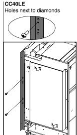
4. Install 2 x part C's onto parts A & B respectively, identify the holes to be used, attach to the unit with 2 screws each.
