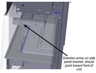
5. Lift up the side panel with the supplied glass clamps (see procedure on previous page). Tilt the side of the glass panel inward and lift up and underneath the upper side panel and hook the 2 outer hooks on to the pins, there is also a panel angle adjustment bracket for the third hook.
