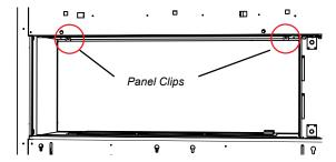
4. Install panel clip into the slots at the top of the side panel as shown.
