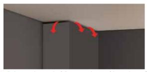
The ventilation opening may be fully open at the top of the enclosure. This type of ventilation opening would be used when the top of the enclosure is not visible from above and where the ceiling within the room is higher than normal. When creating this type of ventilation opening, measures should be into place to avoid having objects of any type falling or be thrown into the ventilation opening. Mesh screen or other preventative measures should be put into place.
