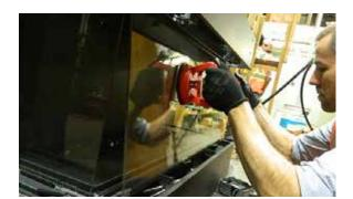
Handle front panel with supplied vacuum clamps
