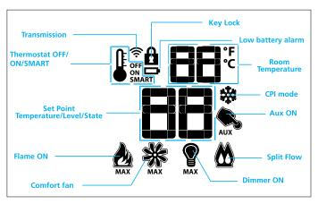
Figure 2: Transmitter LCD Display
