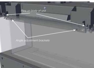
Note: If the outer safety glass panels do not sit at 90° and angle too far inward or outward, remove the glass panel and adjust the screw of the panel angle bracket. Turn the panel angle bracket screw in 1/4 increments—reinstall panel to check.
