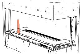
2. Install panel clips into the slots at the top of the back panel as shown.
