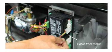
6. If unable to access this Cable - undo 2 screws securing the IFC Board and slide out of unit to access cable.
