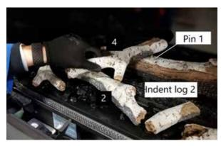
12. Place Log 5—identify the pin locator and match with the right side pin on Log 1. Rest the Log 5 on the indent in Log 3 as shown below.
