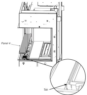
9. Install outer side base panel (5) — panel 5 rests on the tab of panel 4.
