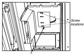
Vent restrictor location - inside top of firebox Diagram 1
