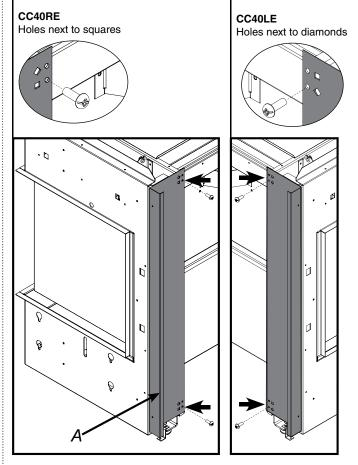
NOTE: CC40LE use holes corresponding with diamond shape. CC40RE use holes corresponding with square shape.
