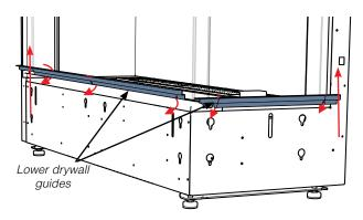
Loosen and tighten screws on drywall guide from inside front panel
