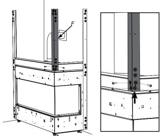
10. Identify G and attach to back corner C and front corner F with 2 screws on each side.
