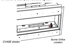
Remove pilot retainer clip with pliers and pull off the pilot cap to expose the pilot orifice.
