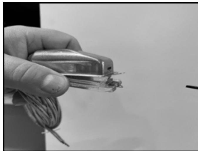
Figure 35: Twist to open glass lens.
