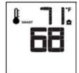
Figure 12: Smart flame function set low.
