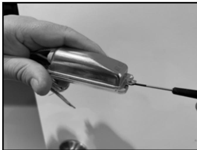
Figure 34: Insert small flat screwdriver.
