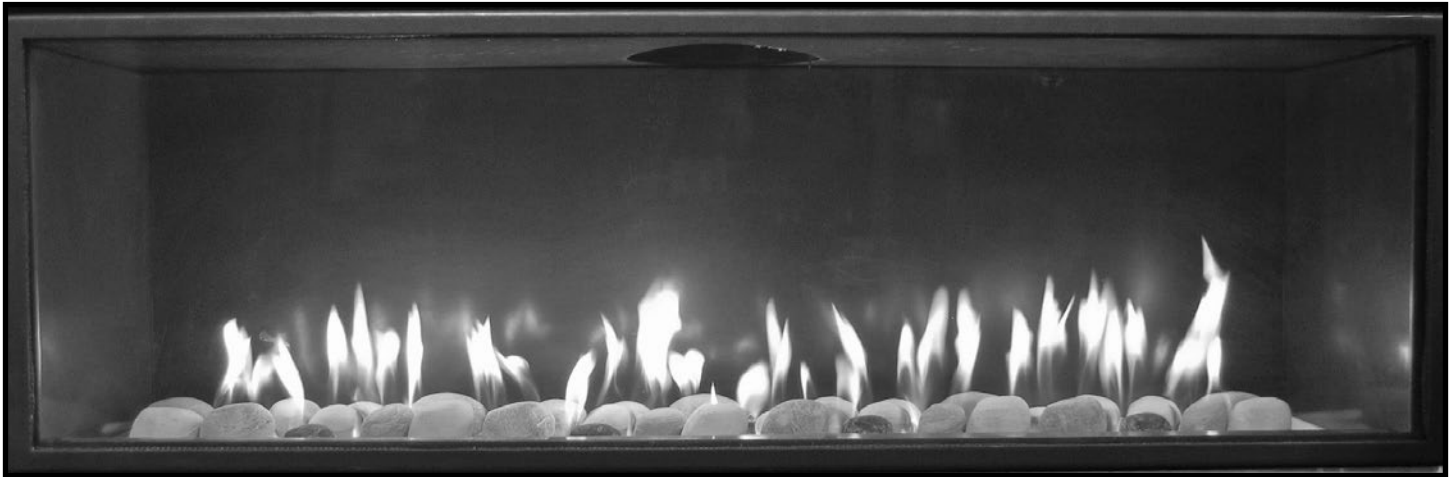
Figure 95: Example of desirable flame pattern.
