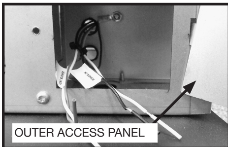
Figure 23: Junction box wiring.
