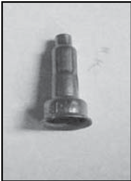
Figure 26: Orifice for propane conversion.
