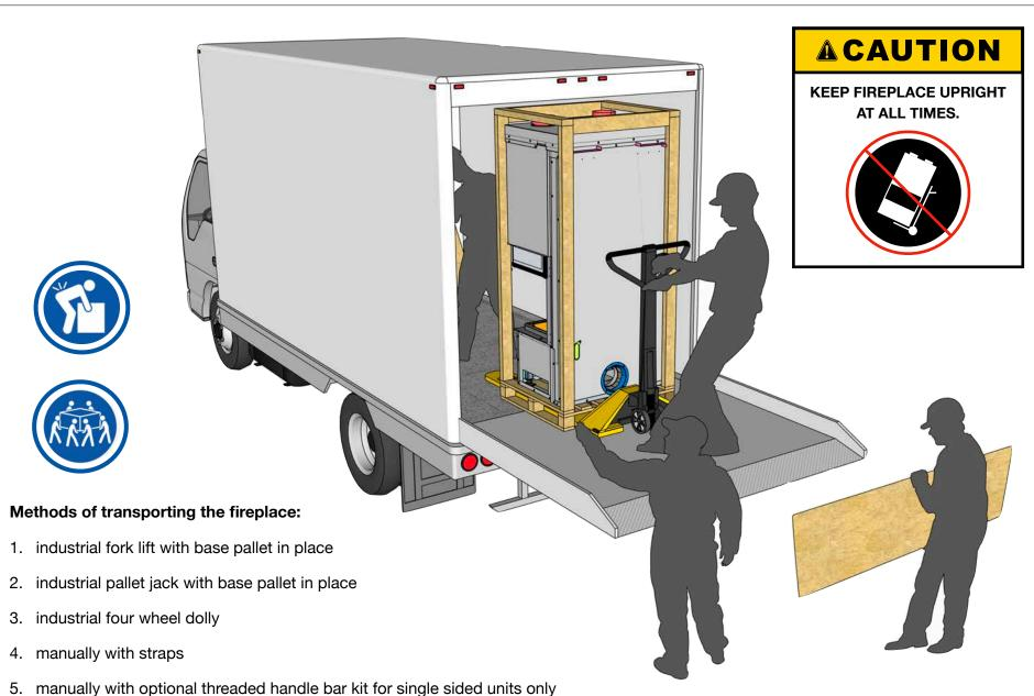
There may be instances when the upper sections of the shipping crate must be removed in order to facilitate moving the unit with height restricted vehicles; through building doorways; making turns in closed quarters; navigating stairways; fitting into elevators, etc.
