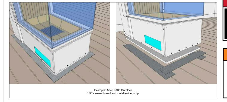
Only non-combustible framing members shall be used to construct the internal framework.
