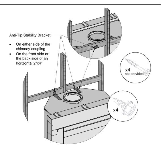
FIGURE 7 ANTI-TIP BRACKET INSTALLATION
