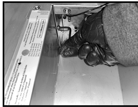
Figure 25: Releasing gas valve assembly from main body.
