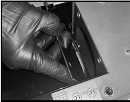
Figure 24: Removing burner cover plate.
