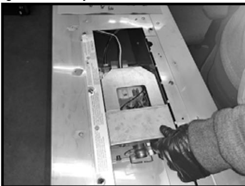
Figure 28: Removing gas valve assy.
