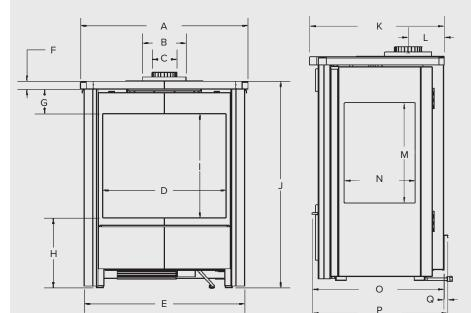
MINIMUM CLEARANCES A 27 1/8" TO COMBUSTIBLES: 36" from front of unit 15  $\frac{1}{2}$ " from side of unit 2 <sup>1</sup>/<sub>2</sub>" from back of unit F 11/4" ALCOVE INSTALLATION: H 11 5/16" I 16<sup>15/16</sup>" 48" depth (max.) J 33 1/2"
