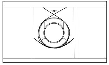
Figure 7.8 Securing Horizontal Pipe Sections
