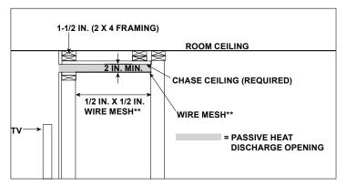
**WARNING!** Risk of Fire! Wire mesh required on bottom of discharge opening when discharge opening is greater than 3 inches. Secure mesh to top of framing.
