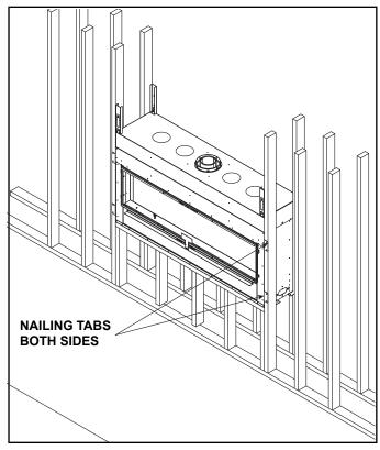
Figure 6.8 Proper Positioning and Securing of an Appliance
