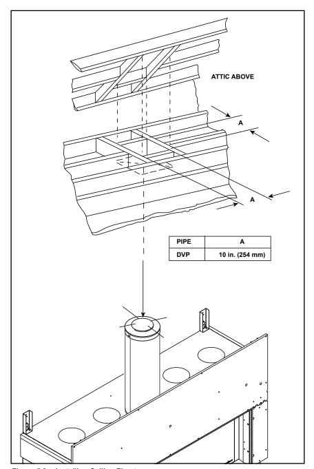
Figure 5.3 Installing Ceiling Firestop
