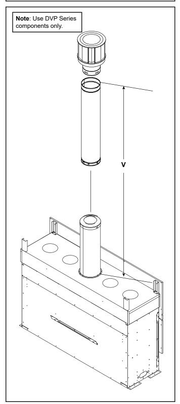
Figure 4.14 Vertical Vent Maximum
