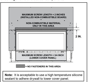
Figure 10.1 Screw Length Requirements
