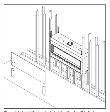
Figure 6.9 Install Factory-Included Non-Combustible Facing Material
