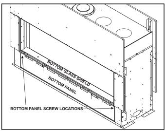
Figure 9.2 Bottom Glass Shield and Bottom Panel Location
