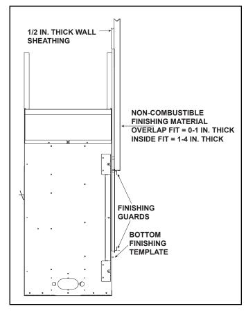
Figure 10.2 Finishing and Facing Materials - Single-Sided Models
