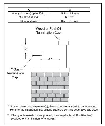
Figure 4.2 Staggered Termination Caps
