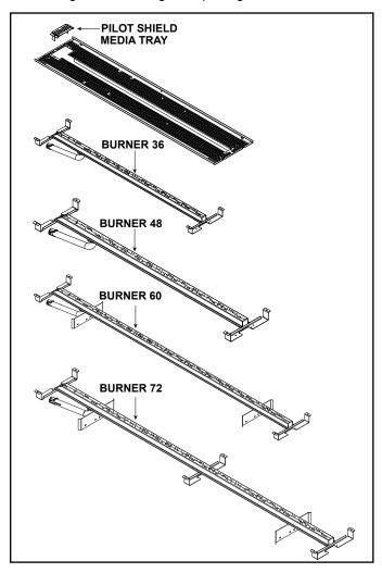
Figure 9.3 Media Tray with Burner and Pilot Shield
