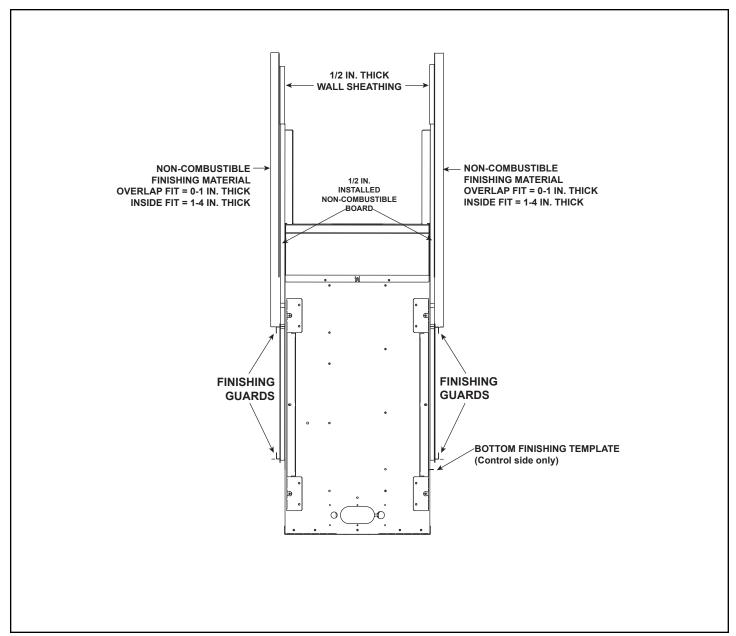
Figure 10.3 Finishing Materials - See-Through Models
