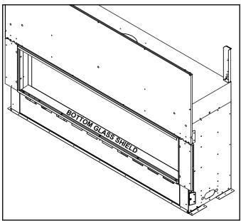
Figure 11.2 Bottom Glass Shield Location
