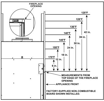
Figure 2.1 Good Faith Wall Surface Temperatures Above Appliance (CRAVE4836-C/CRAVE4836ST-C/CRAVE6048-C/CRAVE6048ST-C)
