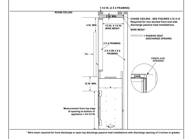
Figure 10.19 Clearances with Passive Heat Optional Heat Management System Installed
