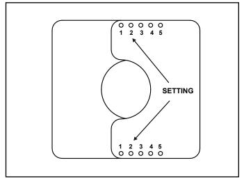
Figure 4.17 Set the Exhaust Restrictor
