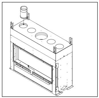
Figure 6.5 Heat-Zone-Gas Linear Adapter Collar
