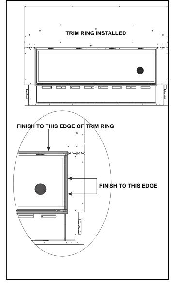
Figure 10.7 Non-Combustible Finish Material Diagram for 1-4 Inch Thick Inside Fit Method Using Trim Ring (Option #2)
