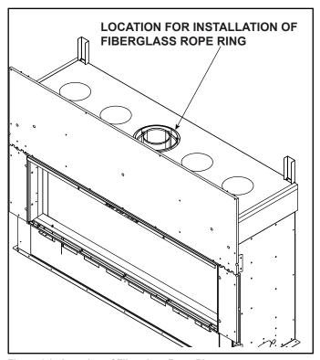
Figure 6.3 Location of Fiberglass Rope Ring
