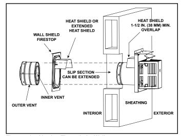
Figure 7.14 Venting Through the Wall
