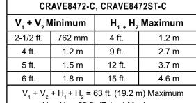
$H_1 + H_2 = 23 \text{ ft. } (7.1 \text{ m}) \text{ Maximum}$
