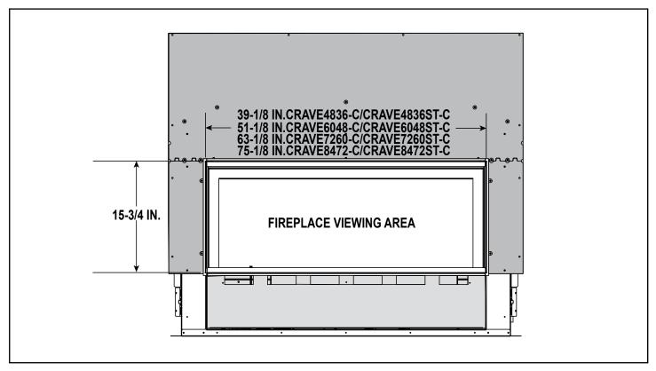
Figure 10.4 Minimum Finished Opening Dimensions - Clean Face Trim Front Method
