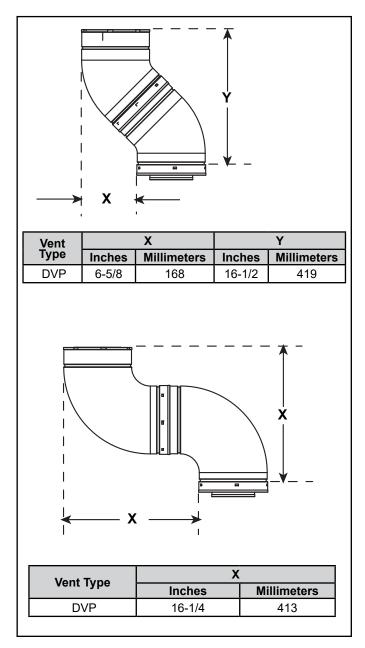
Figure 4.7 Vertical and Horizontal Offset for DVP Elbows
