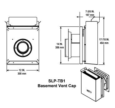
Figure 12.5 Vent Components
