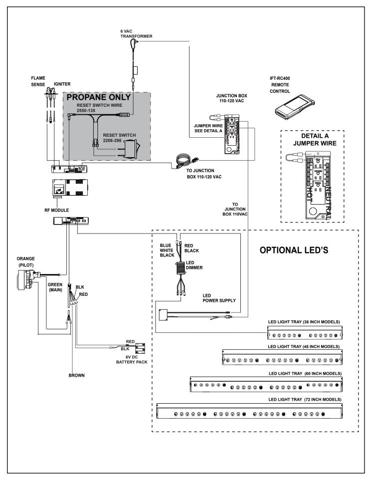
Figure 8.4 IntelliFire Touch Wiring Diagram
