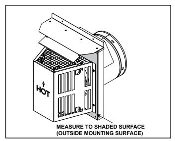
Figure 4.9 Measure to Outside Mounting Surface
