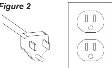
**⚠ DANGER:** Improper connection of the equipment-grounding conductor can result in a risk of electric shock. Check with a qualified electrician or serviceman if you are in doubt as to whether the product is properly grounded.
