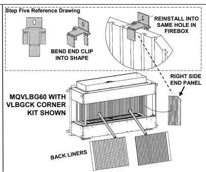
**STEP FOUR:** Install Lower Liner Clips [x3]. Reinstall Media Fence as shown, with one row of slots exposed.
