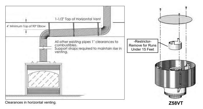
Clearance to perpendicular wall 24 inches (60 cm). (Recommended to prevent recirculation of exhaust products. For additional requirements check local codes.)
