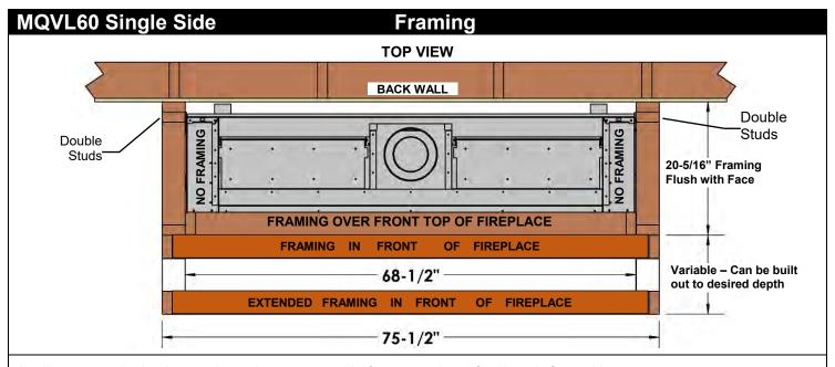
Appliance must be in place with venting connected before area above fireplace is framed in. Fireplace Chase MUST BE VENTED with or without grills.
