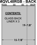
NOTE: Install MQVL48RGB Before installing MQVL48RGE End Panel Kit. STEP ONE: Remove Liner Clip and screws from inside of firebox with a 1/4" hex driver. Discard Back Clip but **Keep Screws**.
