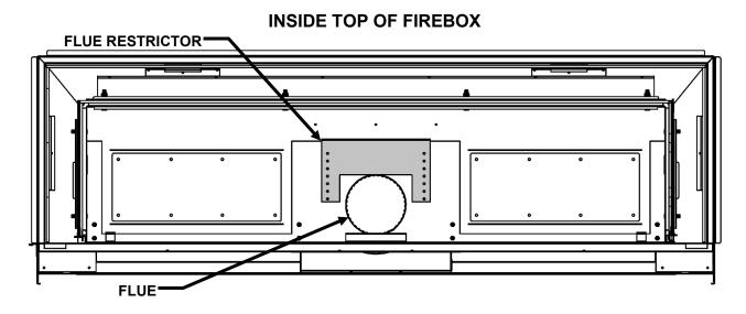
To adjust the Flue Restrictor, remove DT Screws from the firebox top and install the Flue Restrictor over the flue, partially blocking it. **Replace ALL DT Screws.**
