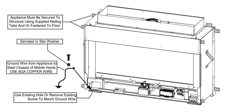
THE VENTED GAS FIREPLACE HEATERS (ANSI Z21.88) IN THIS MANUAL MAY BE INSTALLED IN MANUFACTURED (MOBILE) HOMES AFTER FIRST SALE IN THE USA.
