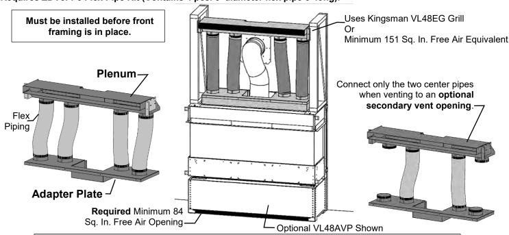
If using insulation in vented chase (i.e. for outside wall), wall board / drywall is required to support all insulation. Vented chase must be clean and free of all debris (i.e. loose insulation, pieces of wood, etc.).
