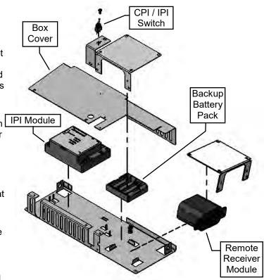
**NOTE:** The Remote Receiver module can also be located outside of the appliance to a maximum of 6ft away installed in a certified deep wall switch electrical box (2-3/4" depth). For this configuration an extension wiring harness (P/N: 1001-P904SI) is required.
