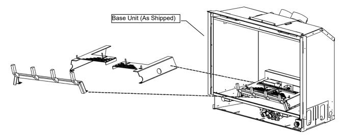
**Preparation**: Remove Grate Bar and replace screws. Remove Ember Plates. Do <u>not</u> remove existing Pilot Shield. **Installation**: Place MQRSP4 or MQRSP8 over burner.
