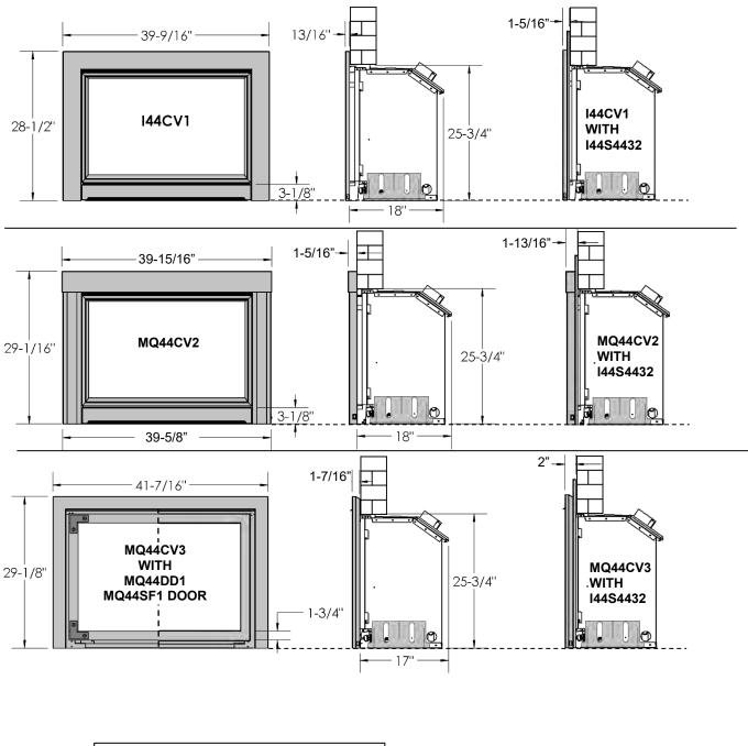
NOTE: Clean View Hooks are adjustable (1/4") for uneven wall surface.
