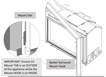
Position the Clean View assembly onto the Backer Surround, align the four [4] screw holes, and fasten in place. CAUTION: AVOID EXCESSIVE PUSHING ON SCREWS.
