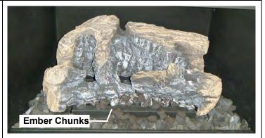
A bag of **Ember Chunks** is supplied with the appliance. It is very important that these chunks are placed onto the front burner and log mounting pan as shown in the picture. Spread the Ember Chunks out no more than one layer deep.
