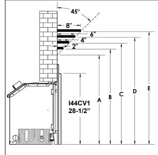
**WARNING:** Combustible objects must not be placed on a non-combustible mantel unless the non-combustible mantel meets the minimum height and width requirements for a combustible mantel.
