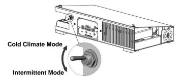
This appliance may run with the pilot continuously running (cold climate mode) or in intermittent mode. For most homeowners, the intermittent mode is preferred (as this saves fuel). However, in some situations the homeowner may prefer to switch the appliance to cold climate mode. The most typical reasons for switching to cold climate mode are:
