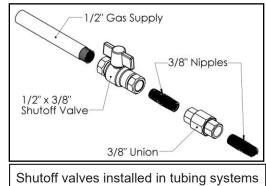
Shutoff valves installed in tubing systems shall be rigidly and securely supported independently of the tubing.
