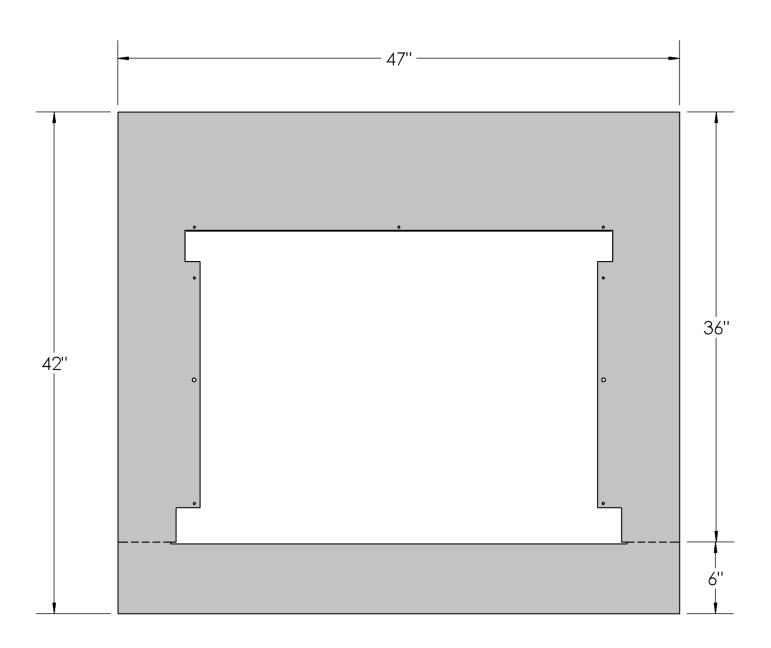
Cut Surround at dotted line shown above to make the bottom flush with the fireplace bottom.
