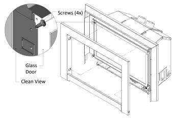
4 Install the Safety Screen assembly onto the Glass Door. This is done by first aligning the lower tabs into slots located in the Glass Door. Then position the upper Screen Hooks onto the upper Glass Door Slots. Push down to engage hooks as shown in the illustration on right.
