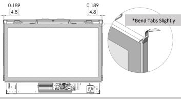
\*RECOMMEND: Slightly bend the two [2] upper door tabs (~10°) as shown above to help ease installation of Safety Screen. DO NOT OVERBEND.
