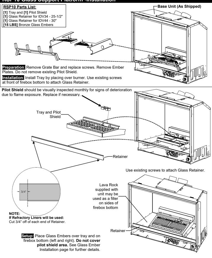
WARNING: Failure to position the parts in accordance with these diagrams or failure to use only parts specifically approved with this appliance may result in property damage or personal injury.
