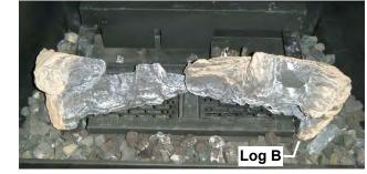
**Log B** has 2 locating holes. Position those 2 holes over the 2 pins on the right side of the log mounting pan as shown in the picture above.
