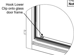
To install screens hook bottom clip onto glass door frame, then press down and push upper clip under top glass door frame, then release. Clip will hook onto frame.
