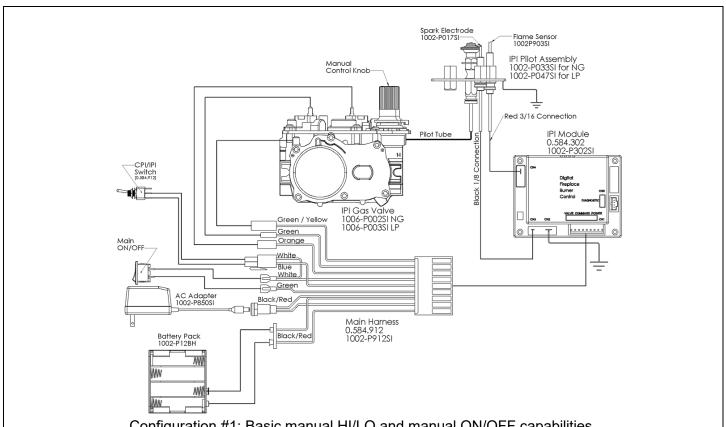
Configuration #1: Basic manual HI/LO and manual ON/OFF capabilities.
