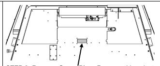
STEP 2: Remove *Cover Plate*. Remove old sealant. Insert Lamp Wires through access hole in firebox. Apply New Sealant (Mill-Pac). Secure Lamp Plate with screws.
