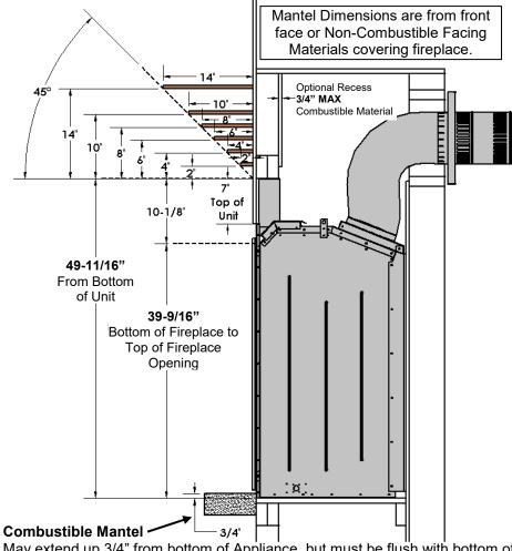
May extend up 3/4" from bottom of Appliance, but must be flush with bottom of fireplace when using **ZCV47S1** Surround or **MQZCVDD** Doors.
