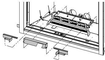
**Step One:** Remove Log Holder, Liner Supports and Screws shown above on side of firebox bottom.
